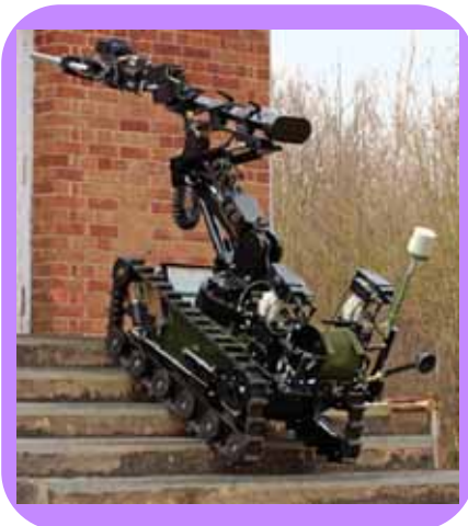
A remote control explosive device disposal vehicle. Photo courtesy of Remotec Ltd
